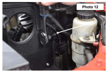
12. Place the threaded isolator in the shield as shown in Photo 13 and secure to shield using the supplied serrated lock nut and washer. Snug nut, do not overtighten using a 10mm socket.
