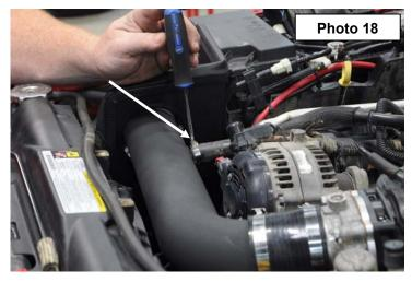
18. Install the supplied hose tie downs as shown to hold the overflow hose in place with factory hardware. Tighten using a 10mm socket. **See Photo 19.**
