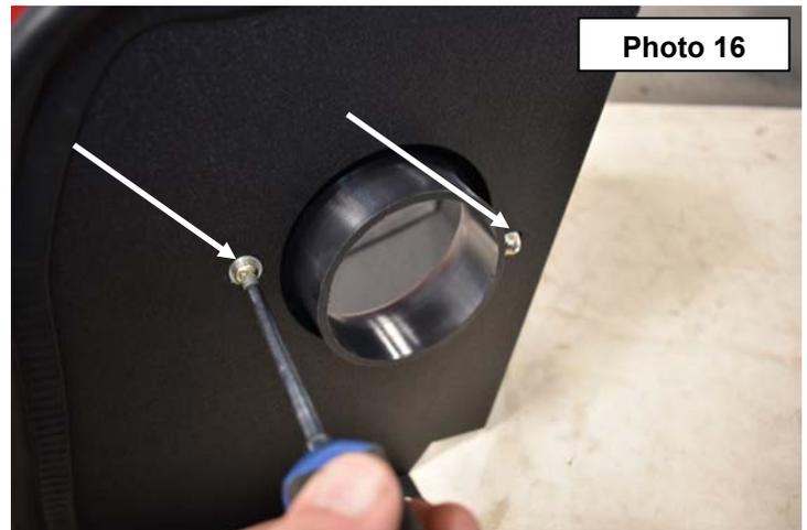
15. Install the cold air intake shield using the factory hardware as shown in the stock air box mount location. Tighten using a 10mm socket. **See Photo 17 & 18.**
