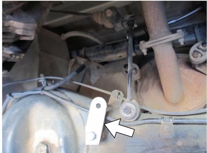
Fit link to relocation bracket using original bolt. Secure with flat washer and nyloc nut supplied.
