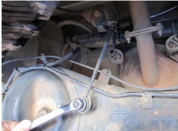
Fit relocation bracket to mount on axle housing with M8 x 20 bolt, spring washer and flat washer supplied.
