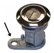
The arm on the back of these lock cylinders are designed to work with 84/90 XJ Cherokee, 86/90 MJ Comanche, 87/90 YJ (tailgate only), and 81/86 CJ-7,8 (tailgate only). In order for these to function on the doors for YJ and CJ models the arm must be removed from the OE lock cylinders and installed on the replacement cylinders.
