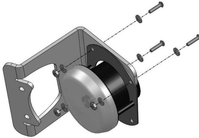
***E. Install the fog light and bracket into the bumper using the remaining two holes available in the light insert. Use the 1-1/2" length 1/4" stainless steel button heads with 1/4" washers and nuts.***
