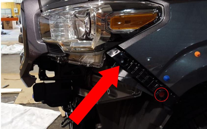
*Remove pin (circled) and remove bolt (arrow) then replace after removing plastic piece*
