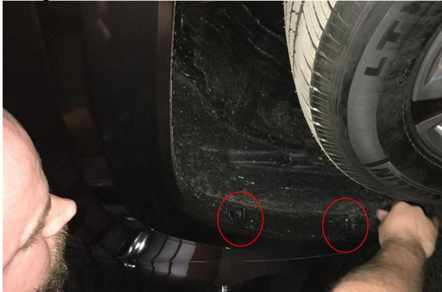
B. Carefully remove the fender flares by starting at one end and slowly pulling away from the truck to tear the tape.
