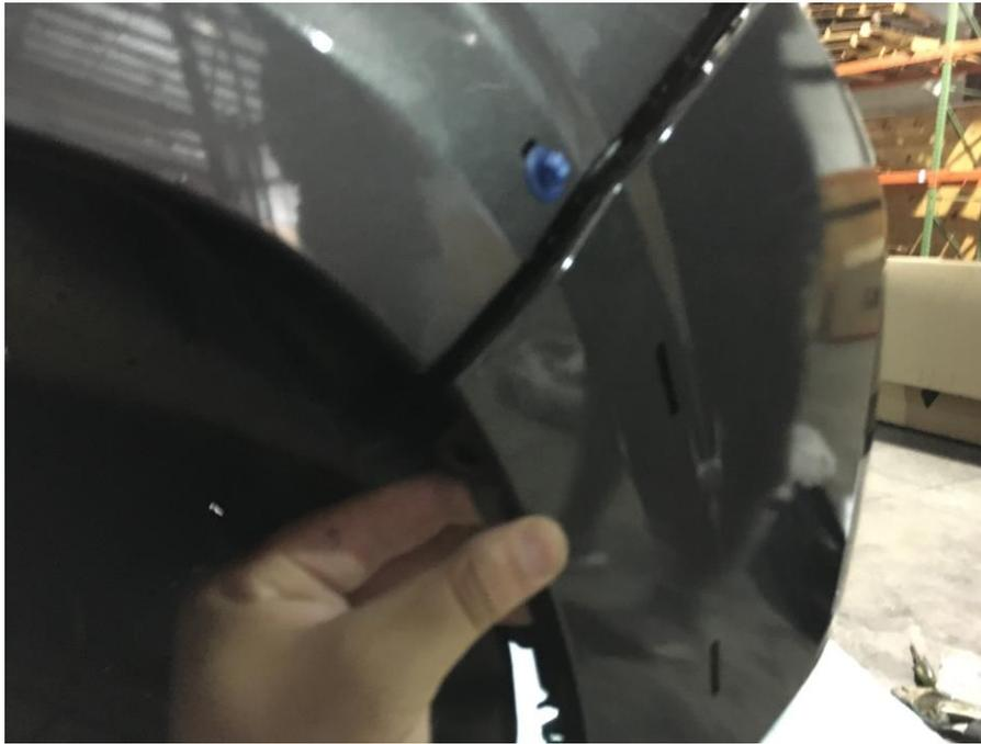
**H.** Remove 2 10mm bolts at the center bottom of bumper.
