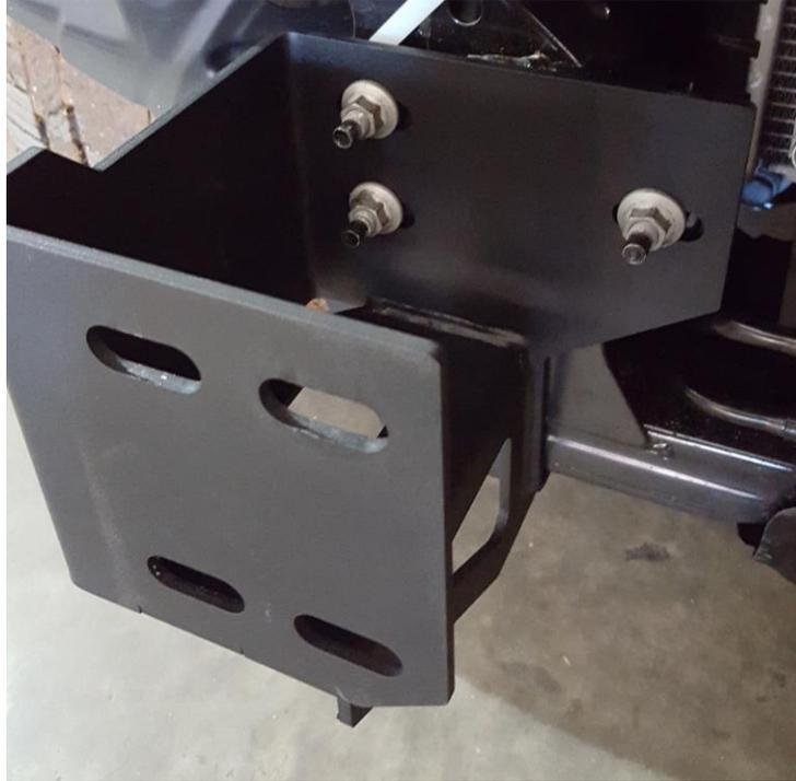
**G. Mount bumper to brackets using the provided 1/2" hardware and stud plates.**
