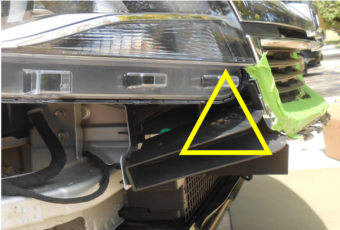
Figure 5d (mount point on plastic grill mount)
