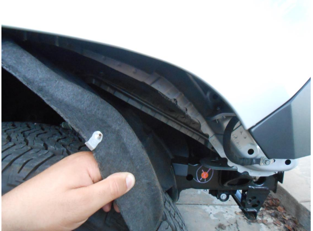
Figure 6a (wheel well liner pull back)
