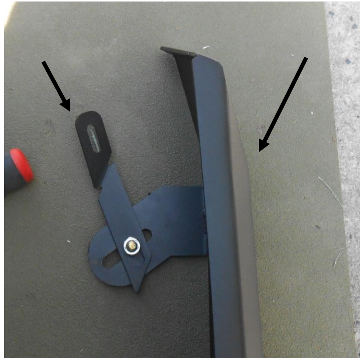
Figure 5a (valence loosely bolted to valence mount)
