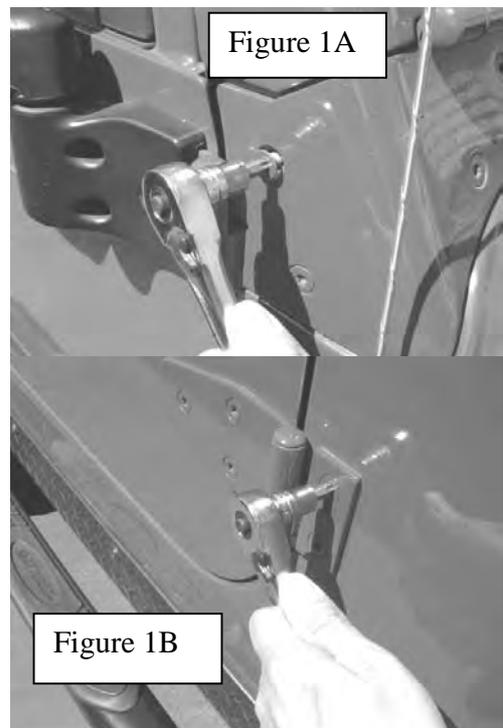
4. Using the supplied front upright 1/4x20 allen bolts and a 3/4" flat washer, attach the front upright to the Jeep. You will need a partner to place the factory backing plate (Figure 2) for the lower door hinge in location for you to attach the lower door bolts. (Do not open the door you are working on! Enter from the opposite side). Tighten the bolts for the upright and repeat the process for the opposite side. (Figure 3)
