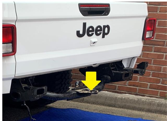
7. If your truck is equipped, remove the four sensors by pushing the housing clips apart and pulling the sensor out. (Figure-7)
