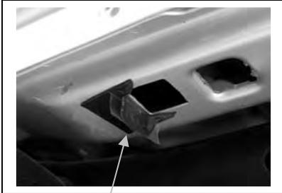
Fig 3. Thin foam adhesive tape. Driver side front
