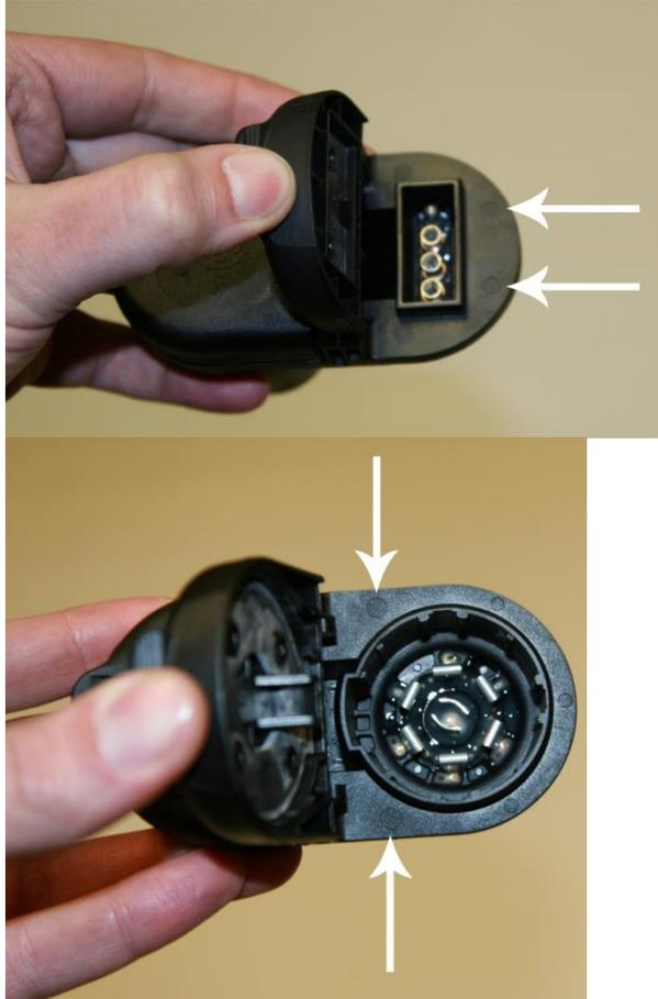
4. Install the trailer plug into the cutout in the new bumper using the #8 supplied hardware.
