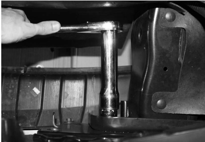
**Figure 2 - BUMPER MOUNTING BOLTS (VIEW FROM TOP)**
