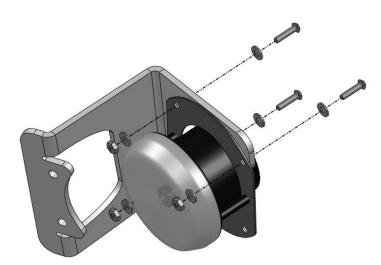
H. Install the fog light and bracket into the bumper using the remaining two holes available in the light insert. Use the 1-1/2" length 1/4" stainless steel button heads with 1/4" washers and nuts.
