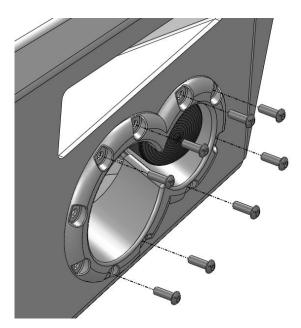
G. Install the Fab Fours fog lights onto the mounting brackets as shown below using the #8 button head screws, washers, and hex nuts.
