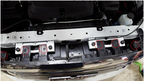
H. Remove the grill and bumper as one piece and detach the grill from the bumper by releasing the clips.
