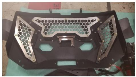
3. If installing an Adaptive cruise control module install module to the included bracket using the provide M8 nuts. Then install bracket to grill section using the 2 lower center insert 5/16" bolts
