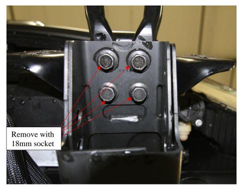
5. Next, using 18mm socket remove the two nuts on either side of the frame attaching frame horns to frame. Set bolt strips and nuts aside as they will be used in the installation of Fab Fours Grumper. (See image.)
