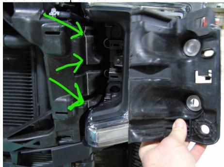
12. If equipped with a front facing camera in the grill remove it at this time using a torx bit and pulling back on the squirter mechanism.
