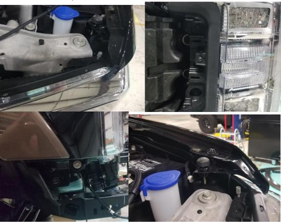
10. Remove the horns saving the oem hardware. Remove all harness clips from the plastic grill support.
