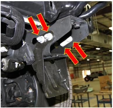
6. Open hood and locate push pins on radiator cover. Using a flat head screw driver, pull the head of the push pins up, remove push pin and lift radiator cover off. This will allow access to top grill bolts.
