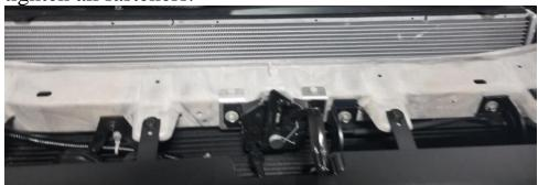
5. At this time if you have a front mount camera install in the grumper from this inside as shown. On the hold down bracket install the included foam on the camera side and trim as shown.
