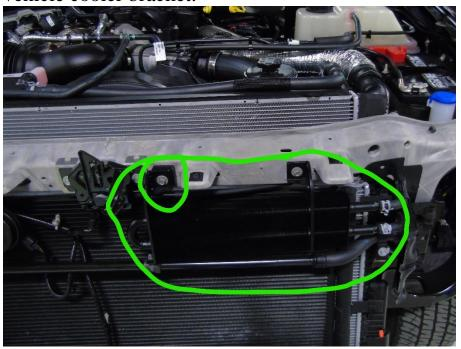
2. Mark using a silver marker the plastic grill support along crease as shown below. After marking on both sides, cut along marked lines.
