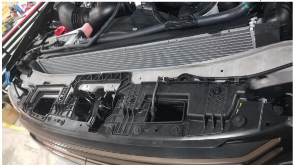
8. If equipped with front camera remove the camera washer Tee from the main washer line and reconnect the main washer line to itself the can be done by pulling up on the black retainer collar.
