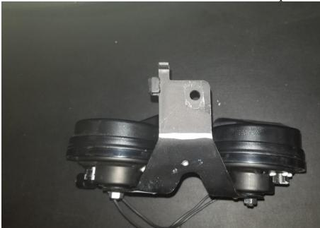
6. Straighten out remaining bend in horn bracket.
