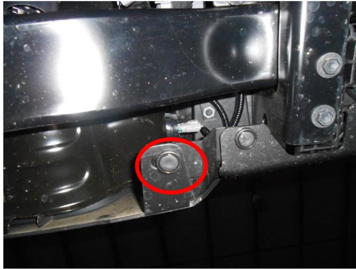
***E. Use a 12mm socket to remove 10 bolts on the metal piece of the lower bumper.***
