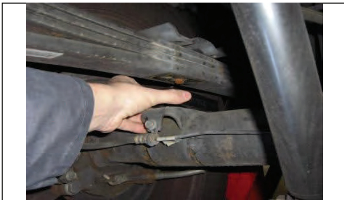
Center lift block on axle pad under leaf spring pin side down.
