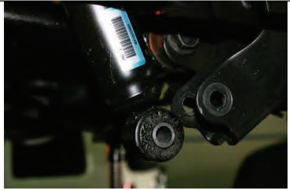
Disconnect rear lower shock from axle mount.
