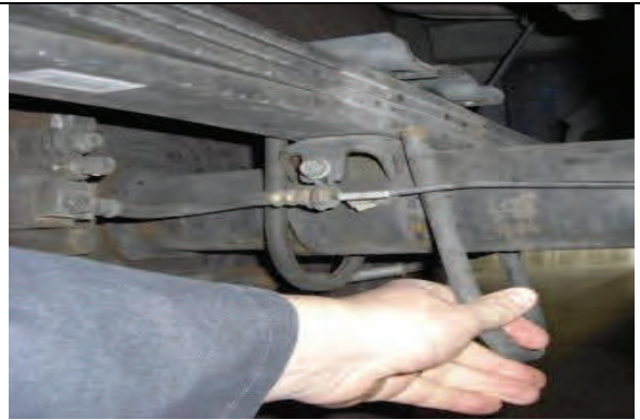
Remove u-bolts and carefully lower axle.
