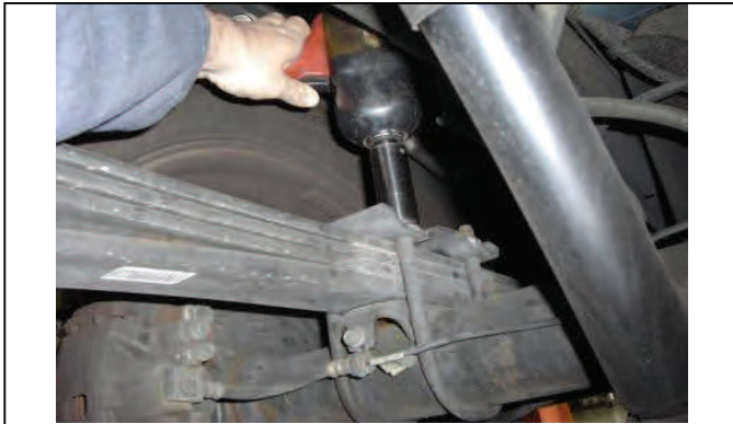
Work on one side of vehicle at a time, remove rear u-bolts.
