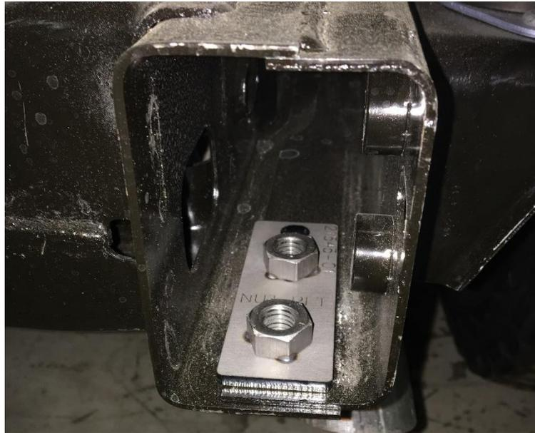
13. With a friend, carefully hold the bumper and swing arm assembly up to the Jeep and use the 1/2" bolts to attach the nut plate along with the OEM side bolts.
