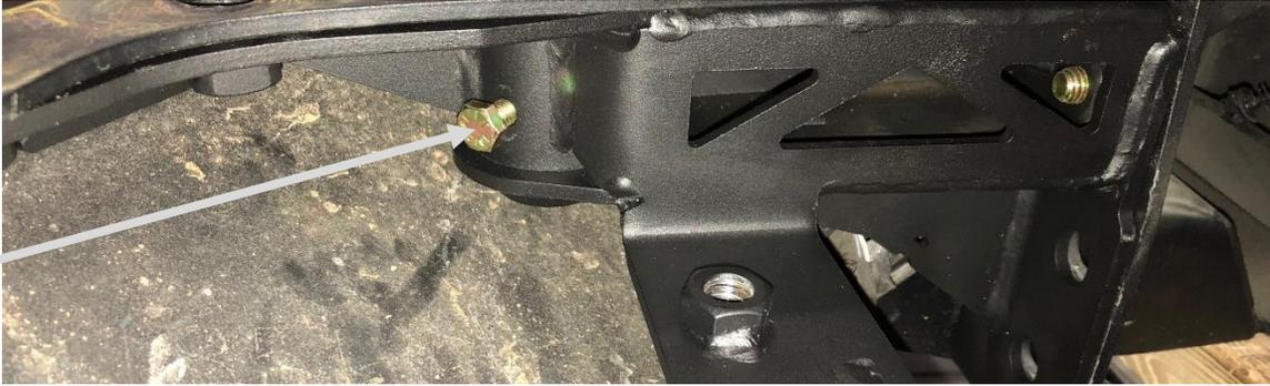
11. Once the swing arm is installed use a grease gun to fill the swing arm cylinder with grease.
