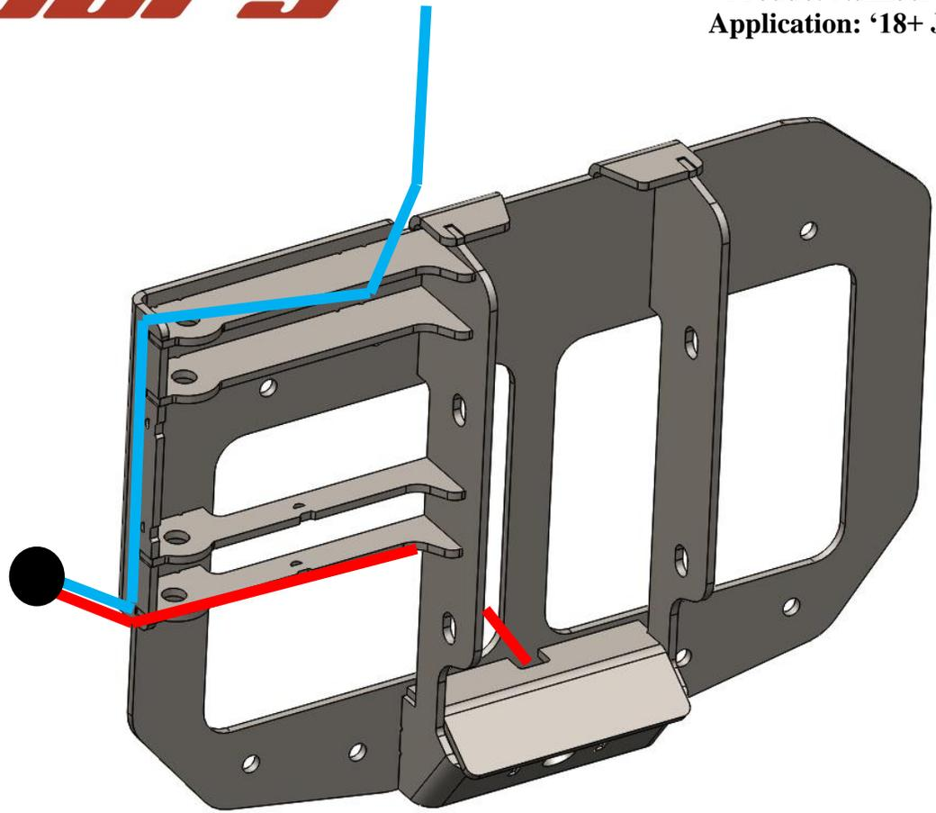
21. Use zip tie holes to secure the harness in place
