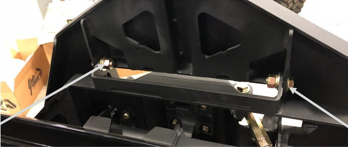
19. Use the  $\frac{1}{2}$ " bolts washers and nuts and bolt through the cradle to the swing arm brackets. (At this point you can chose the desired angle you would like the tire carrier to sit at). Thoroughly tighten all bracketing and mounting bolts at this point.
