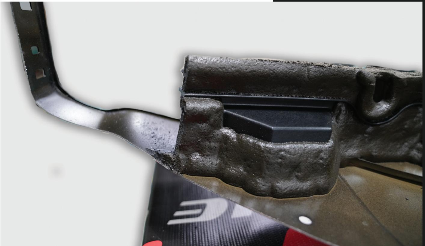
Using a body saw, flip the fender over and cut off the plastic mold along initial cut line.
