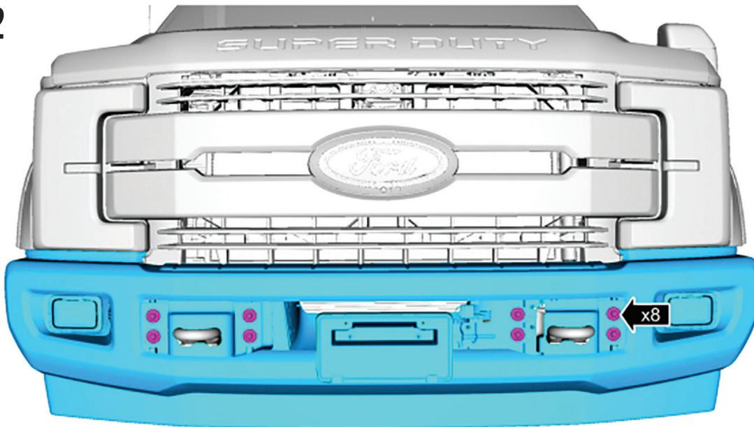
With the help of others, and using an 18mm socket, remove the 8 bolts holding the bumper to the vehicle. Pull bumper away from vehicle.
