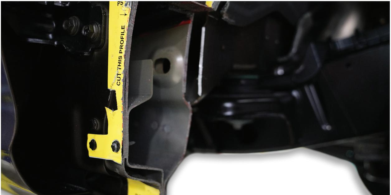
Take care when cutting template 6 cut line. Do not over cut and penetrate the firewall.
