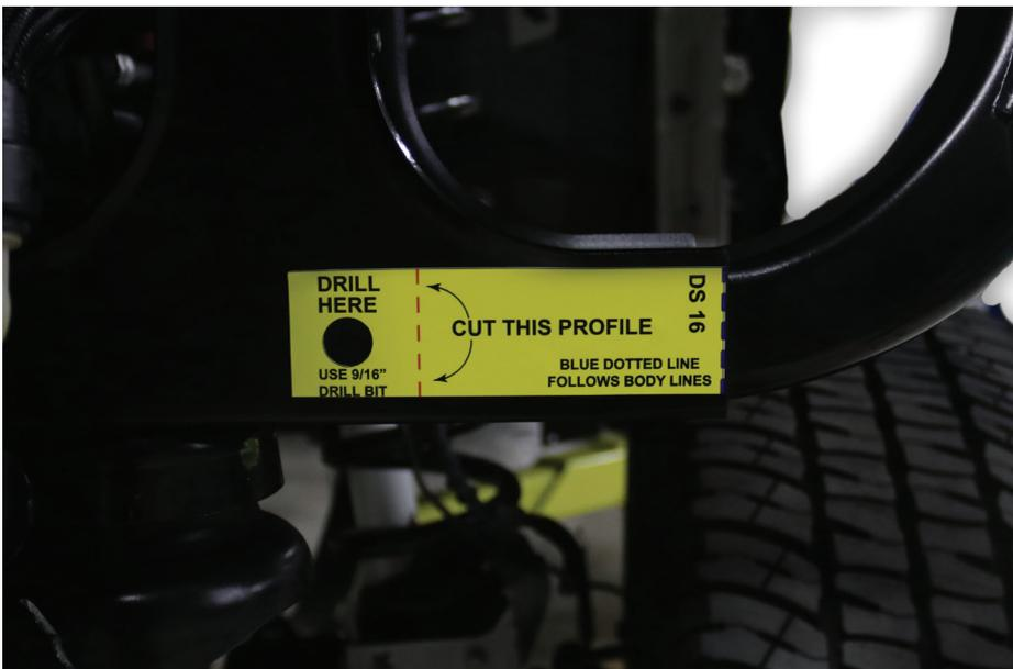
Cut template 16 & 10 is installed by lining the edge of the template up with the edge of the reinforcement and running the bottom of the template with the bottom of the reinforcement where the radius ends.
