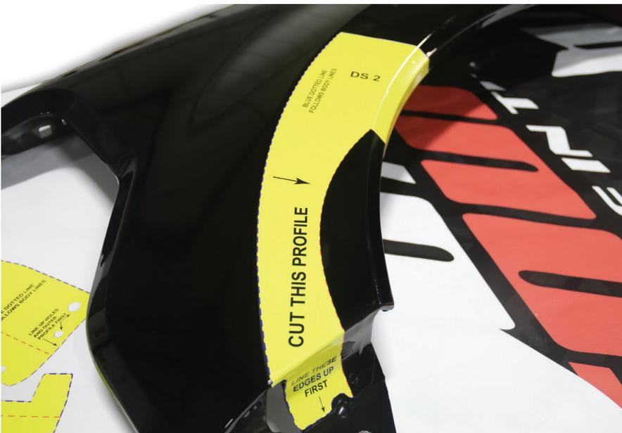
Start by installing cut template 2 on the front bottom edge of the fender of the vehicle. Cut template 2 will be installed by aligning the bottom edge profile with the matching sheet metal of the fender indicated by the red oval. When placing the template, make certain the template is aligned with the contour of the fender, ref purple crescent. Cut template 4 is a mirror of cut template 2
