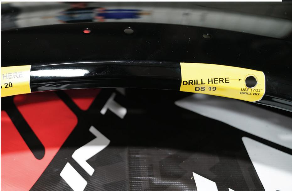
With cutting templates installed you can now drill. Using a center punch and 17/32 bit, mark and drill holes at the locations indicated by the templates.
