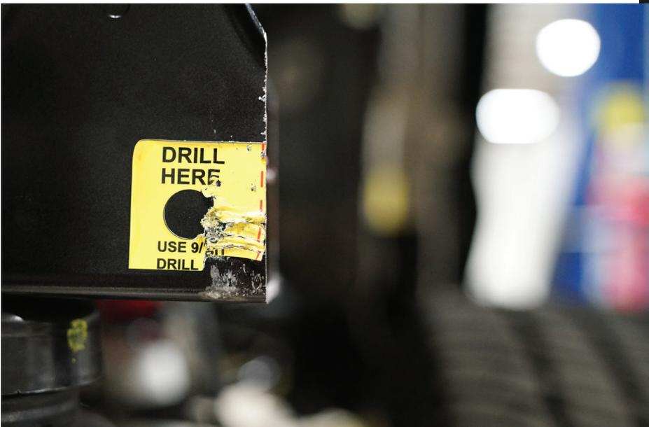
Note: When cutting always error on the side of taking less material away from vehicle.
