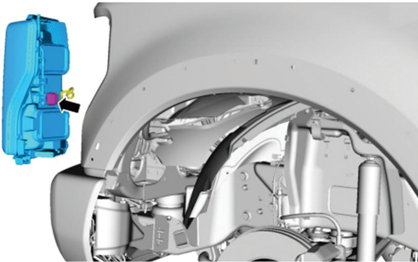
For LED headlight assemblies, disconnect electrical connector as seen in image.
