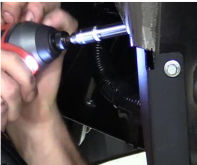
Using a 5/32" bit, drill pilot holes. Reinstall plate on vehicle, using a 3/8" socket and provided self-tapping bolts. With plate installed, tape around edges leaving a gap at the top for the provided foam tube to fit
