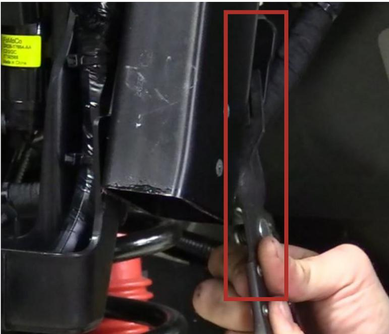
Wiring harness mount will need to be disconnected and floating. To do this remove Christmas trees pin on the inside surface of the reinforcement tube. Plastic housing will need to be floating. To do this remove Christmas trees and using a 10mm socket remove bolt. This will be reattached, using only the 10mm bolt, after.
