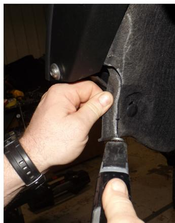
The front OEM inner fenders can be reused with a little modification. Using a small reciprocating saw the plastic/felt can be cut. The profile of the cut is a suggestion and can be modified based upon the opinion of the installer/customer.
