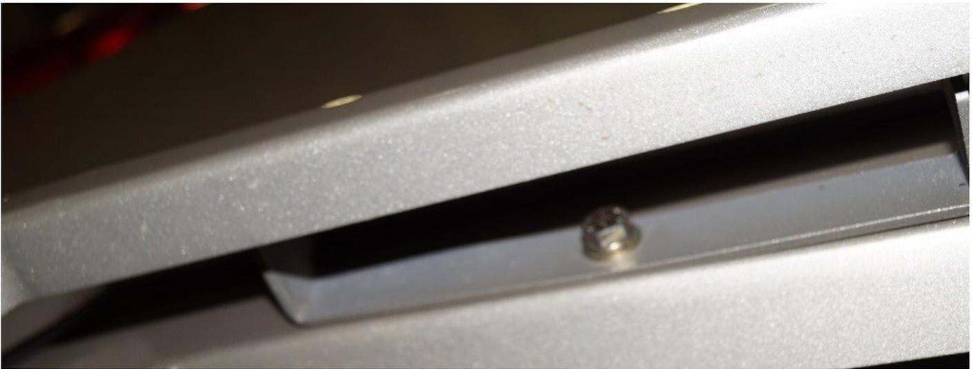
Install seal around edge of fender flare. Using a 1/2" socket/ratcheting wrench, Install fender flare. Install all bolts hand tight. Surrounding images show bolt installation. Leave bolts extremely loose until all bolts have been installed.
