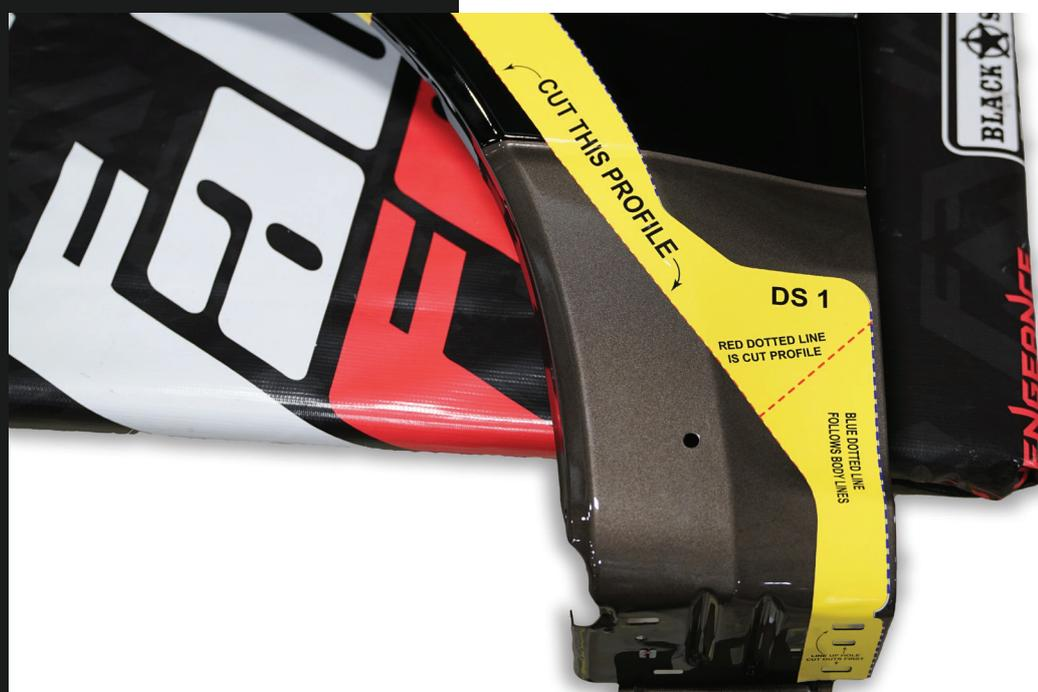
Cut template 1 will be aligned with the holes on the bottom of the fender and the outside contour of the fender. These two areas are indicated by the red ovals in the images around the box.
