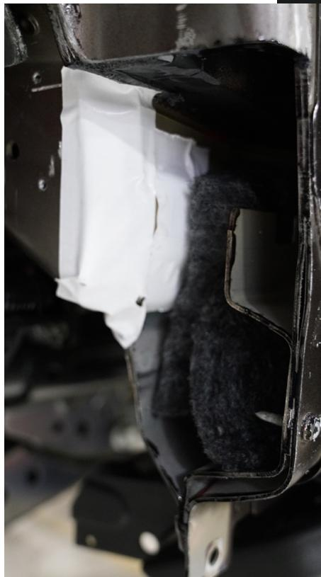
Cut OEM foam straight across 4" from the bottom point. Insert foam into the rocker channel as seen in image on the right. Use duct tape or its equivalent to close off Channel as seen in image on the left.
