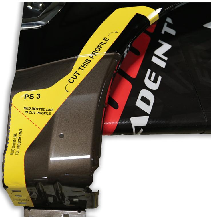
Cut template 3 is the passenger side template and a mirror of the driver side. Repeat steps for Cut template 1.
