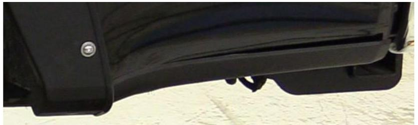
Using shears, cut off the front portion of the kick panels. There should be enough material left to tuck under fender flange. Reinstall kick panels inserting front under fender flange (ref. oval) and using pins to clipping in rest (ref. arrows).
