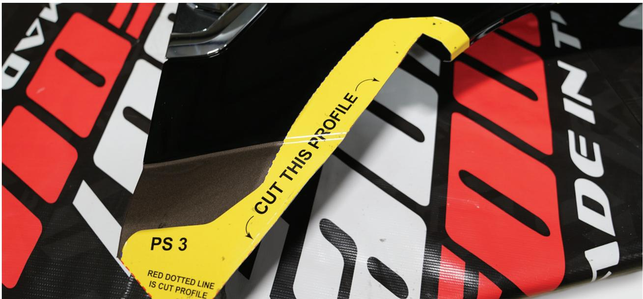
The last step in the front fender cut is to return to cut templates 3 & 1 and to cut off the bottom portion indicated by the red squares. This will remove the rear most bottom of the fender.
