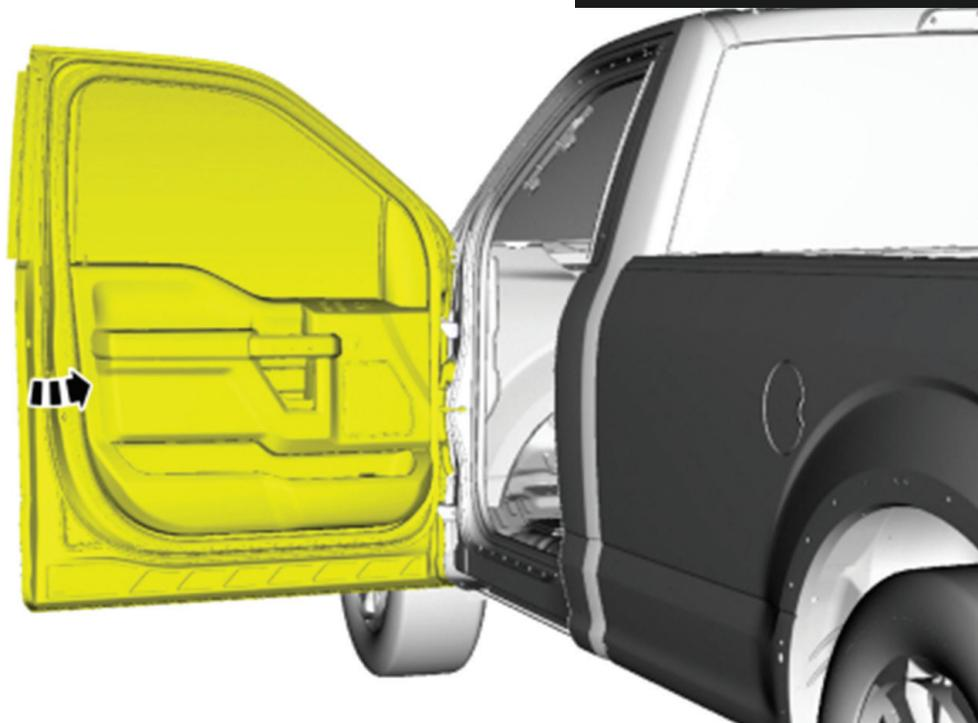
Open the door to gain access to the bolt located in the door jamb toward the top of the fender. Using a 7mm socket remove the bolt. The bolt may have been powdered over making it difficult to grip with the aforementioned socket. Once the bolt is removed close the door.
