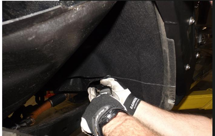
With Felt inner fender installed cut plastic covering to match felt in the back with a larger cut in front.
