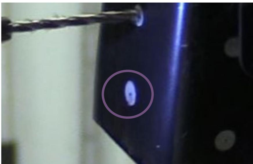
Using a 3/8 drill bit, drill a through hole at the bottom outside hole location indicated by the purple circle to the right.
