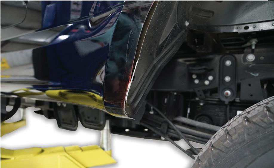
Using saw the final cuts should look similar to photos here on both sides of truck.
