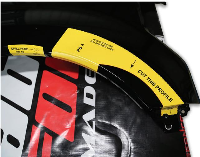
Cut template 4 is the passenger side template and a mirror of the driver side. Repeat steps for Cut template 2
