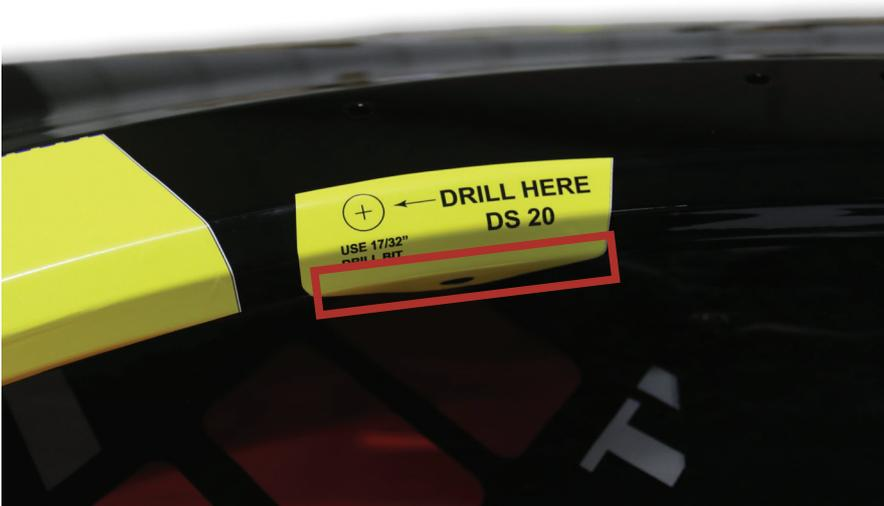
Cut template 20 is mounted by aligning slot and contours at the bottom of the template on the front driver side fender, ref the red rectangle. Cut template 18 is the mirror of above.
