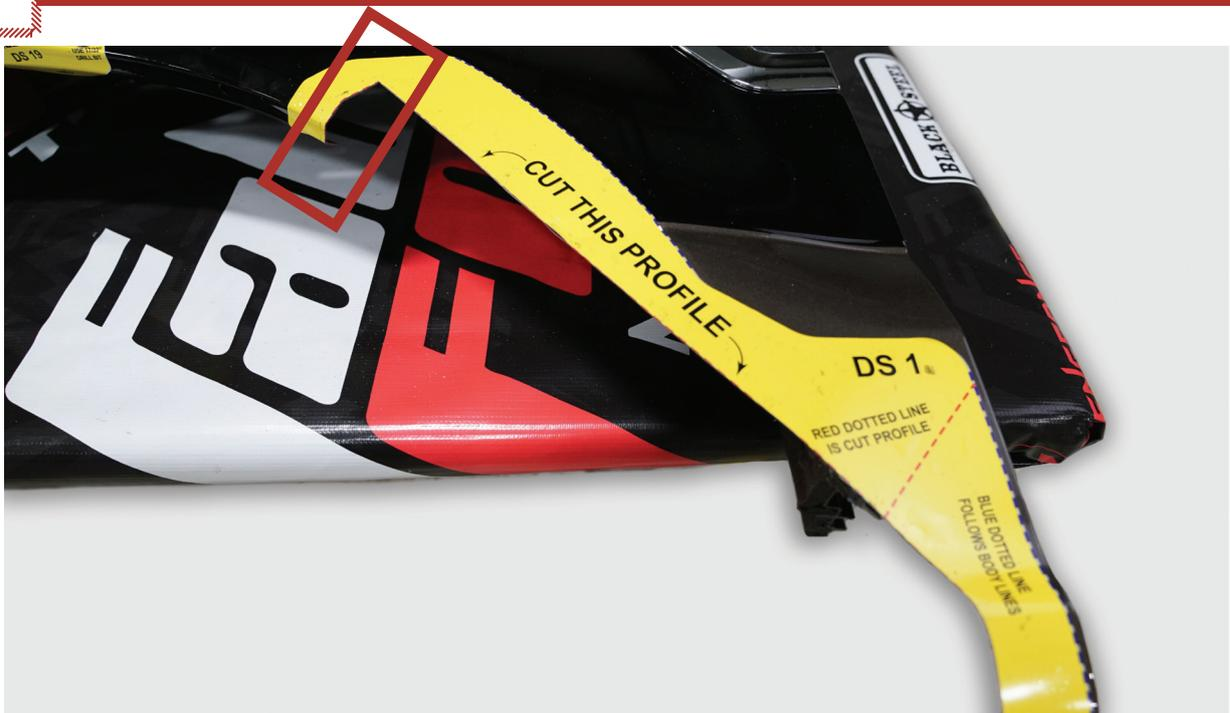
Using a body saw, start cutting the rear portion of fender along the inner most cut profile. Once complete come back and make the 90 degree cuts to meet the initial cut, indicate by the red boxes.
