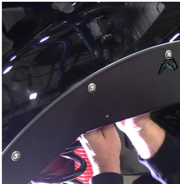
Reinstall the cut OEM foam before reinstalling fender on truck where red square indicates above.
