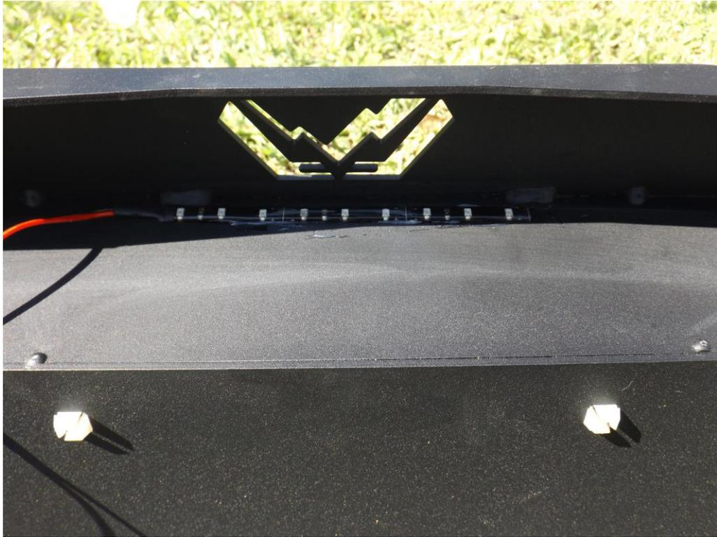
9. Secure all loose wiring and harnesses to the frame or bumper with zip ties.
