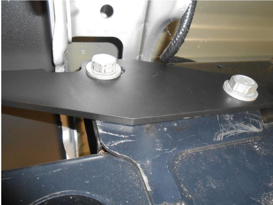
4. Level and align the bumper in relation to the truck bed. Fully tighten all fasteners including bolts attaching hitch bar.
