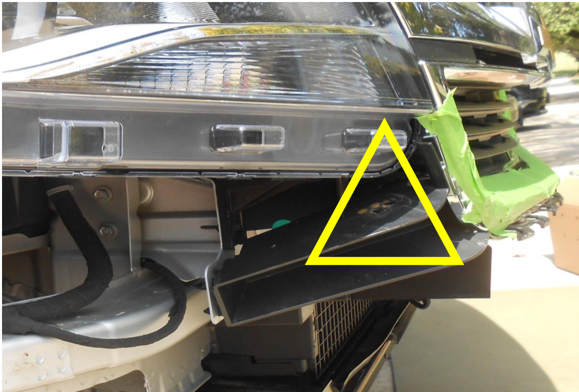
Figure 5d (mount point on plastic grill mount)
