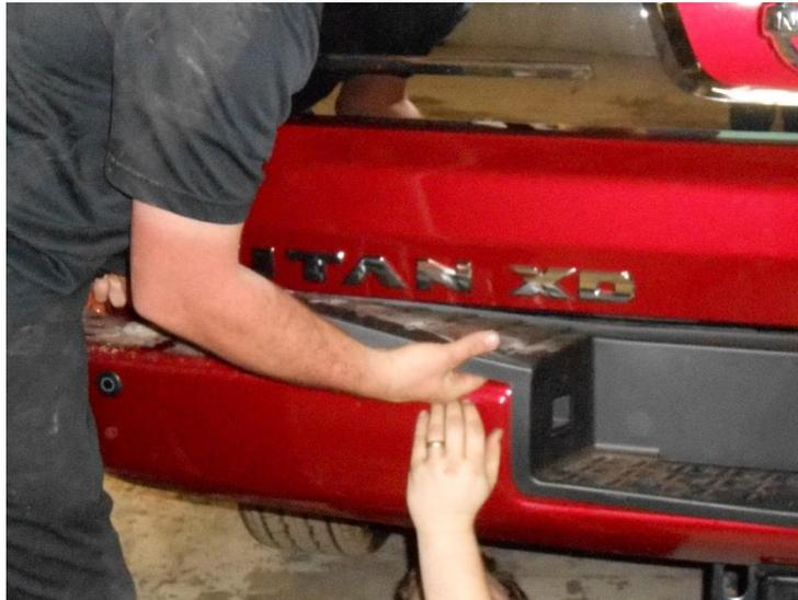
***E. With the help of at least one more person, remove tailgate by removing the limit straps and camera harness from the bed. Then pull up on the driver's side of the tailgate with the tailgate approximately halfway open. Then slide the passenger side off the pivot point. This is at least a two***
