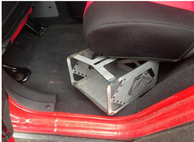
2. Once installed under seat, going through the storage base install brackets by sliding bracket over seat support and starting provided 5/16" bolt into bracket as shown below.
