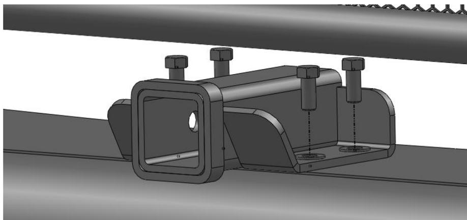
Figure 8 - Hitch Installation
