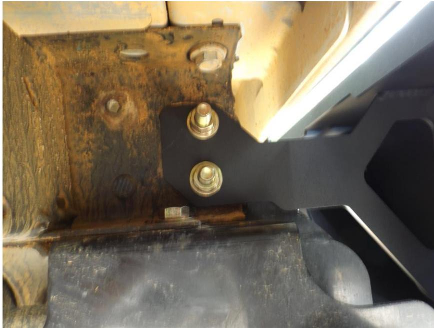
3. Level and align the bumper in relation to the truck bed. Fully tighten all fasteners.
