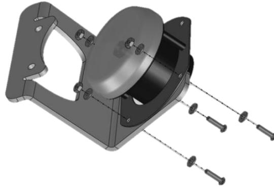
6. Install the fog light and bracket into the bumper using the remaining two holes available in the light insert. Use the 1-1/2" length 1/4" stainless steel button heads with 1/4" washers and nylock nuts:
