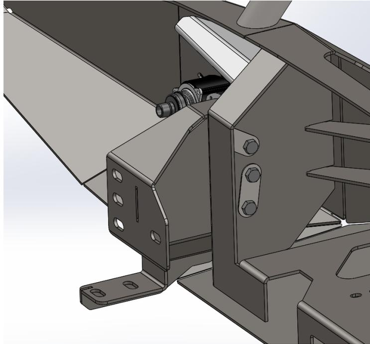
2. Carefully align bumper with intermediate mounts to the frame and slide bumper into place. It may be helpful to support bumper with a floor jack(s) during install. This will at minimum require two people to hold the bumper and a third person to install the supplied hardware.
