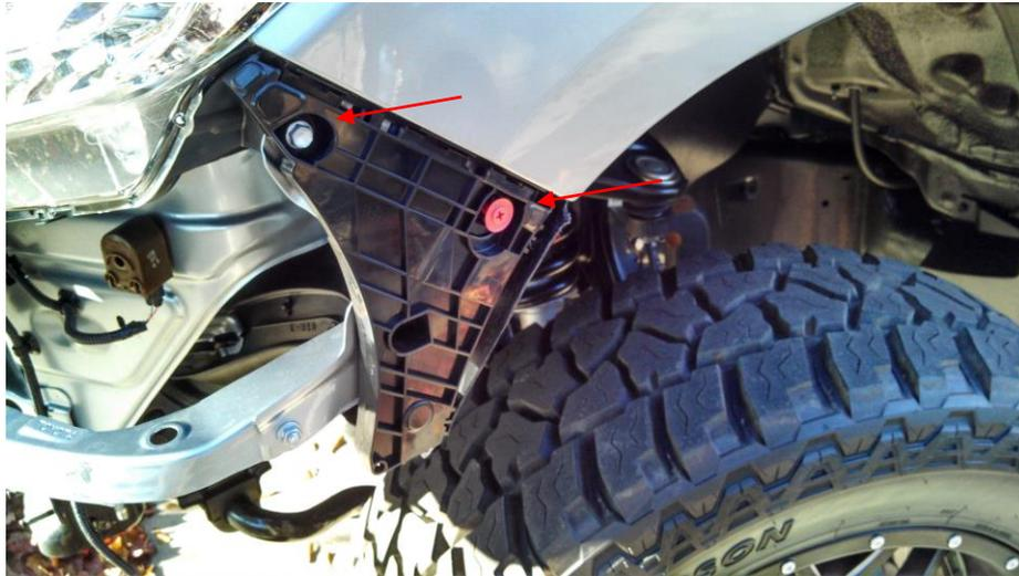
Figure 7 - Spacer Fastener Locations
