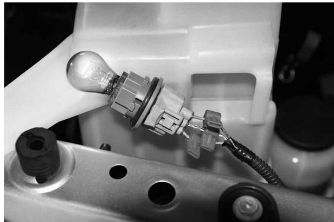
Figure 12 - Turn Signal Wiring Access
