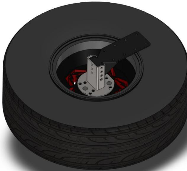
**N. Use the Supplied 7/16"-14 x1.25" Long Bolts, washers(Each Side), lock washers, and nuts to secure the Tire Vertical Mount's channel to the Tire Mount's Channel with two bolts(4 Total) passing through each side and the nuts located on the inside of the Channel of the Tire Vertical Mount.**
