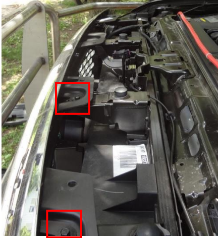
Figure 2a-bolts on LH side
