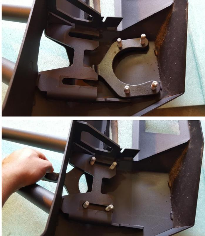
Figure 4: Installing OEM tow hooks
