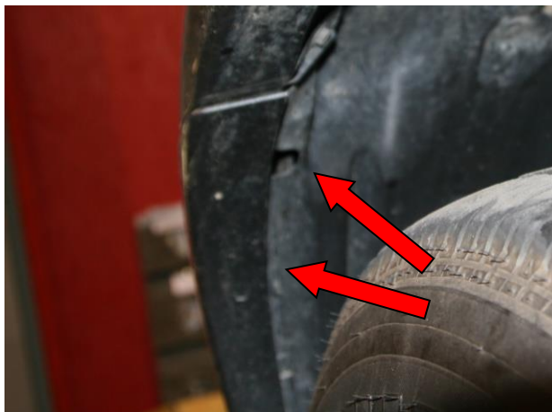
Figure 4 – Fenderwell fastener removal
