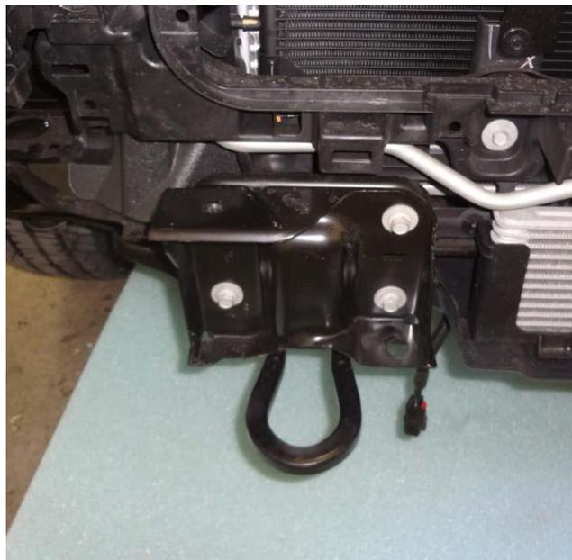
Figure 3b (TOW HOOK & OEM MOUNTING BRACKET)
