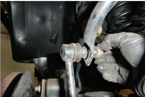
Disconnect and remove rear swaybar endlinks
