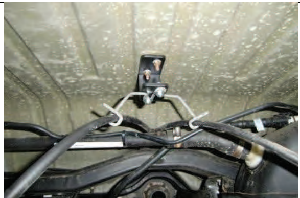
Install provided brake line extension bracket and hardware.
