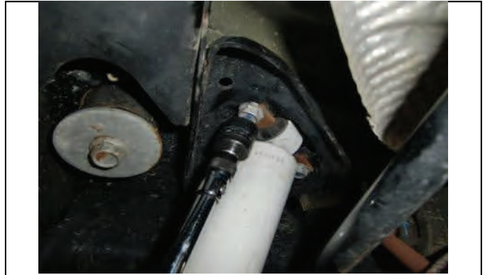
Next, remove rear upper shock bolts.
