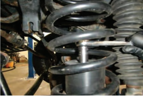
Secure bumpstop extensions to axle with provided hardware.
