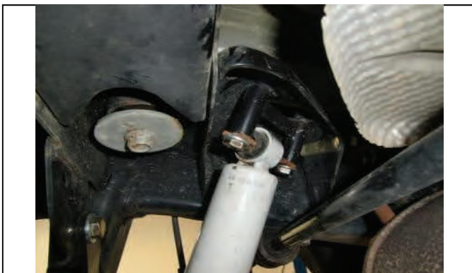
Install upper shock extensions with provided hardware.
