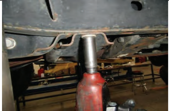
Reinstall front transfer case skid plate bolts.
