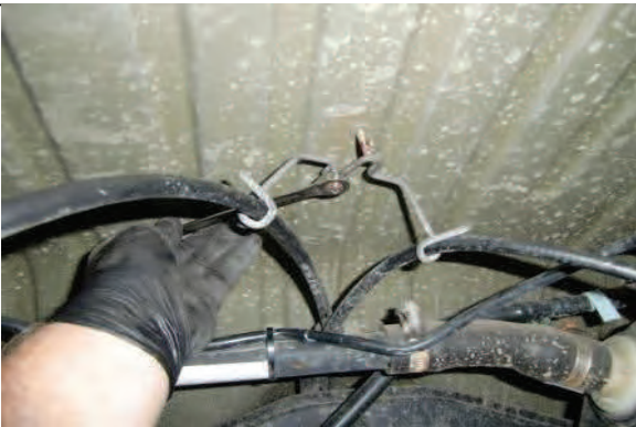
At the rear, remove center brake line nuts under body.
