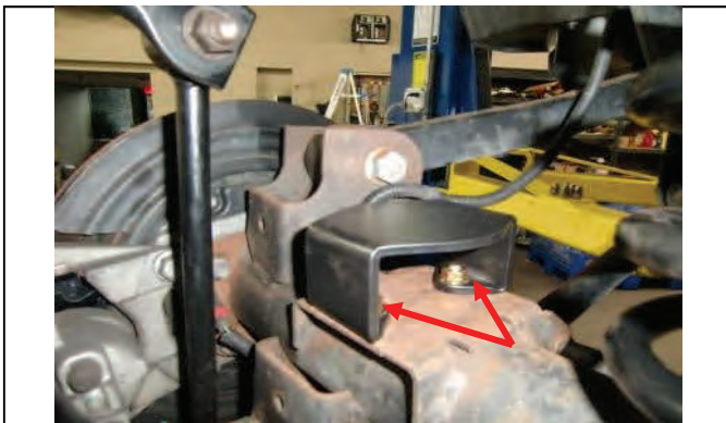
Install rear bump stop extensions with provided hardware.
