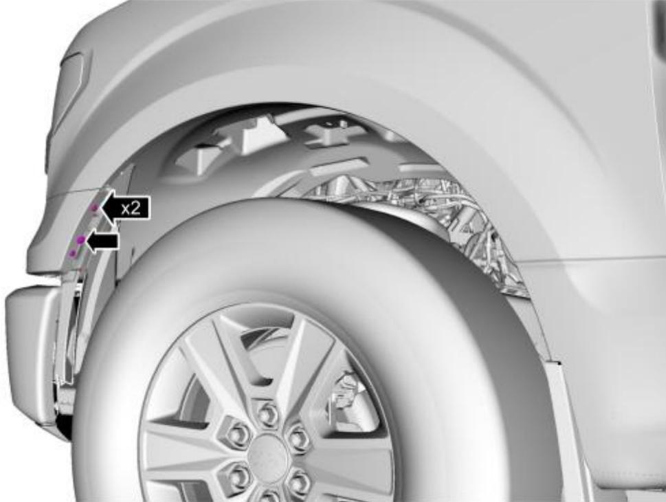
**E. Remove the pin-type retainer.**
