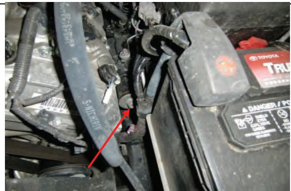
Photo shows UCA mounting bolt and battery proximity
