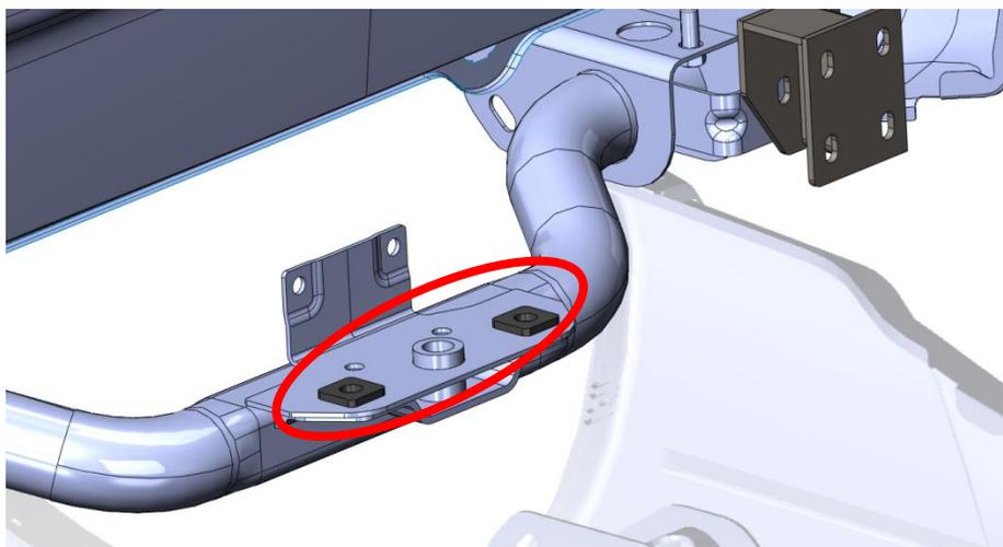
**H. Install bumper mounts onto the frame as shown using supplied mounting hardware: bolts, washers, and nuts. Do not tighten fully. Verify that the angled bottoms on the mounts open down towards the inside. Repeat for other side. See image below.**
