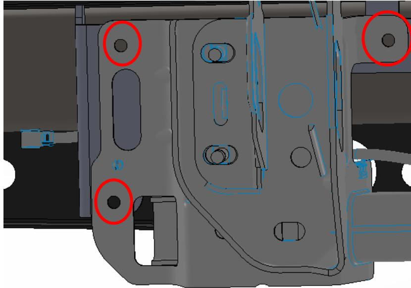
Figure 4 (3x per side, Outer Bolt Locations )
