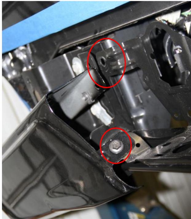
Figure 4b (2x per side, Inner bolt locations)
