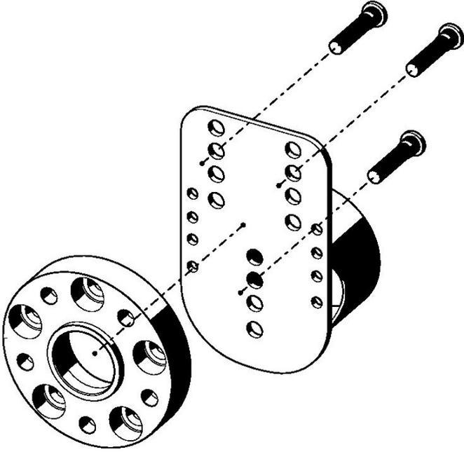
2. After the correct wheel stud holes have been selected, press the new extended wheel studs into the spare tire carrier mount. Slide the supplied wheel spacer over the studs as pictured below.
