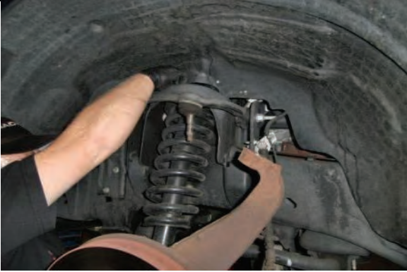
Remove strut upper mounting hardware & remove assembly
