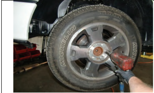
Remove front wheels/tires
