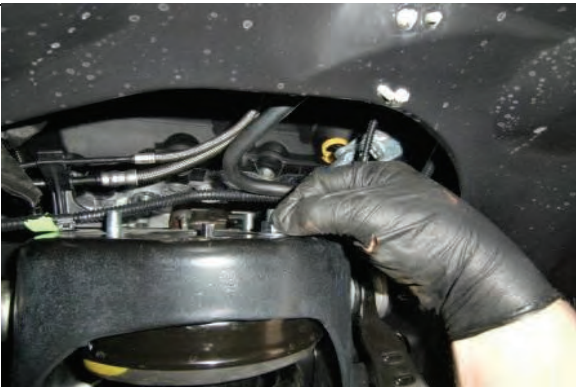
Reinstall strut w/spacer in vehicle w/new hardware, tighten
