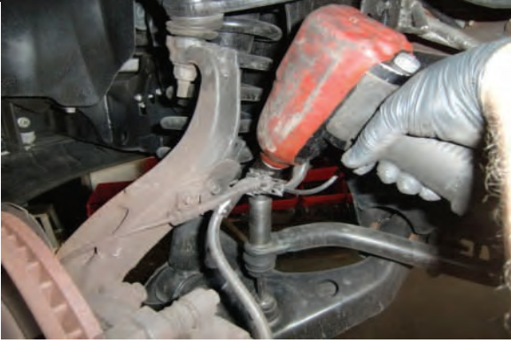
Reattach sway bar end links, tighten to spec
