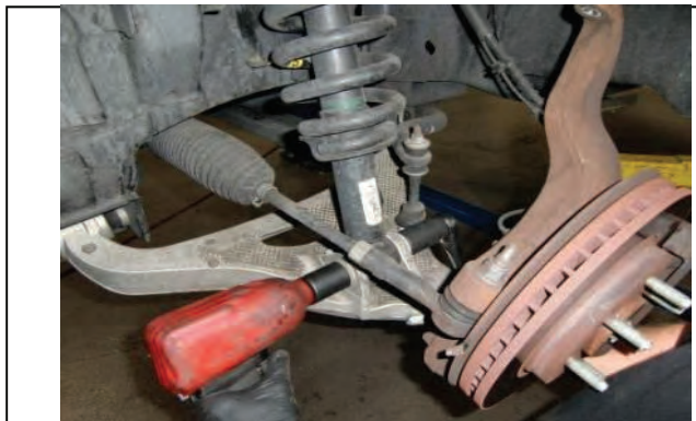
Remove lower strut mounting hardware
