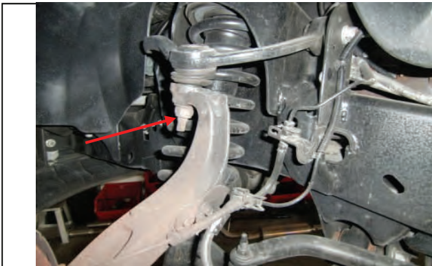
Loosen but do not remove upper ball joint nut
