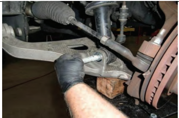
Reattach lower OE mounting hardware, tighten to spec
