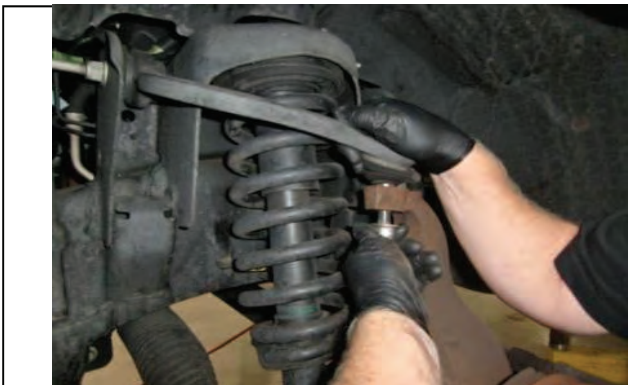
Push down upper control arm and remove ball joint nut
