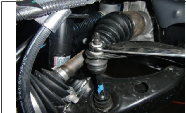
Disconnect sway bar end links on both sides of vehicle
