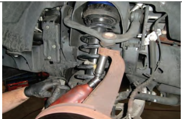
Tighten upper ball joint nut to spec
