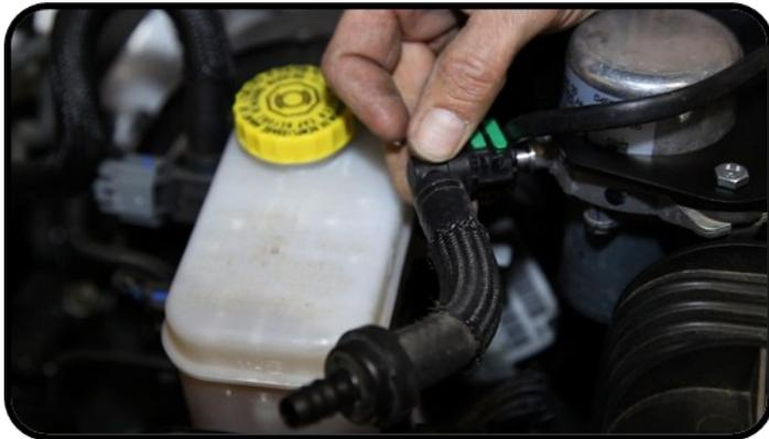
12. Install the 90 degree vacuum connector/hose/check valve into the end of the hose that remains connected to the intake manifold.
