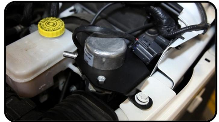
7. Re-install the bolt through the bracket into the fender.
