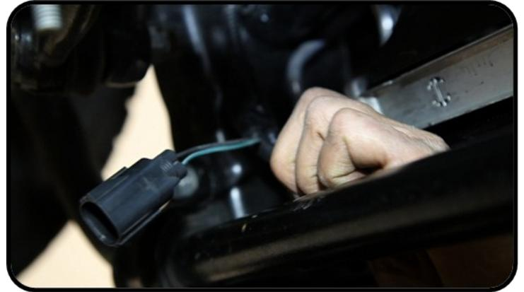
16. Strip 3/8" of the insulation from the two wires protruding from the factory connector and attach the supplied green and black wires to the factory connector using the supplied heat-shrink butt connectors.
