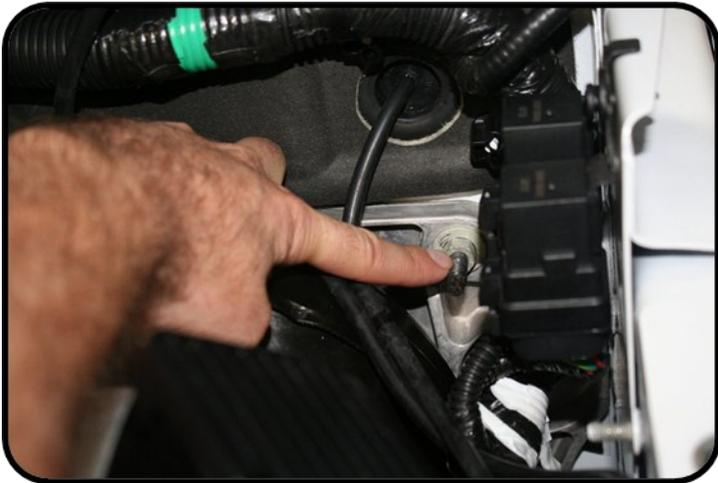
6. Install the horn with bracket onto the stud as shown, re-install the factory nut, and attach the electrical connectors.
