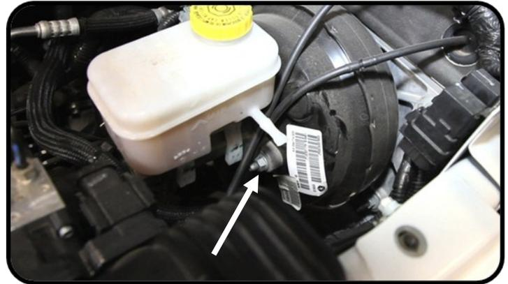
6. Position the pump/bracket assembly such that the hole in the bracket lines up with the threaded fender hole as shown, and slide the slotted portion of the bracket behind the previously loosened nut and over the stud.
