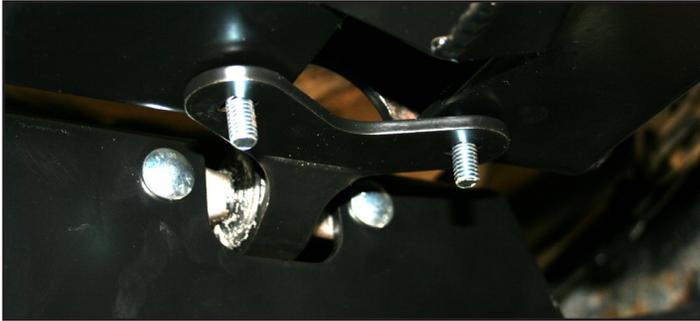
Note: If you are installing the HD engine skidplate at this time you can put the bolts in from the bottom to maximize ground clearance and prevent the nut/bolt from any potential damage.
