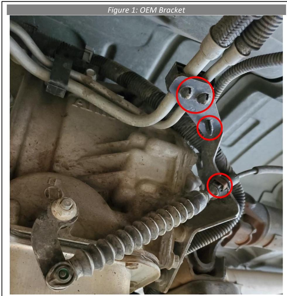
2. With all the wires, hoses, and shift cable loose from the cable bracket, remove the two bracket mounting bolts and OEM bracket. See figure 2. One of the mounting bolts is not visible in the image.
