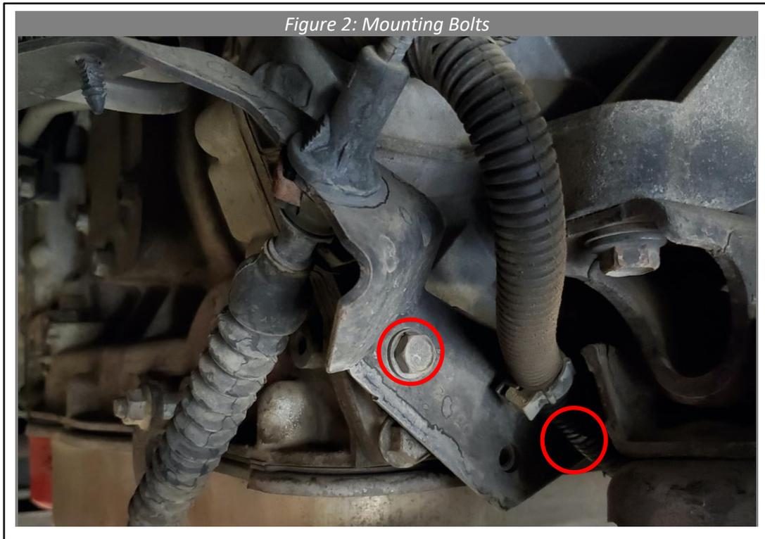
3. Using the 2 bolts removed in the previous step, install the Cognito Bracket just as the OEM bracket was installed. Reinstall the shift cable, safety clip, hose-stays, and wire-stays removed in step 1. See figure 3
