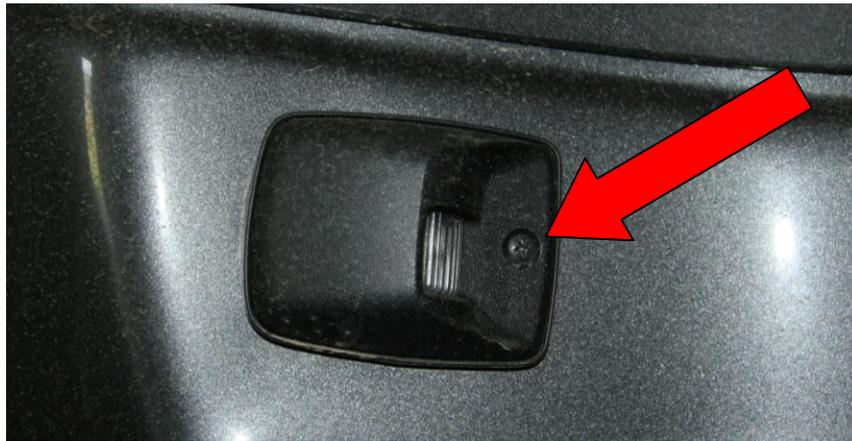
**Figure 1 – License plate light removal**
