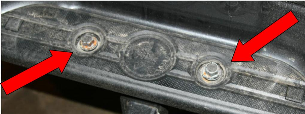
**Figure 3 – Trailer hitch bolt removal**
