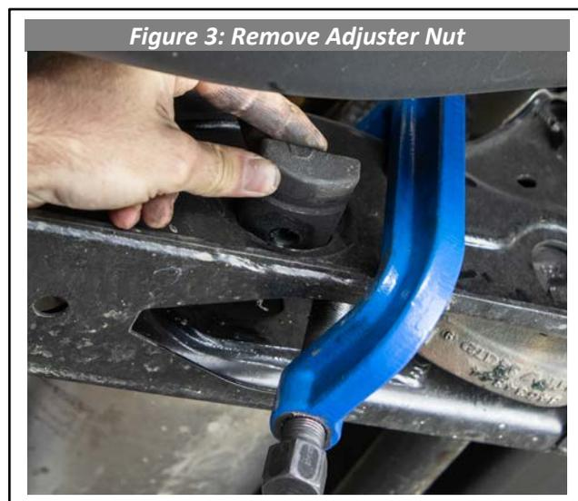
5. Suspension torsion bars hold a lot of energy and both sides of the front suspension are connected through the sway bar. If one torsion bar is loaded, it will affect both sides of the suspension. Unloading them both first is safe practice if other components effected in the front suspension are being worked on or replaced at this time.
