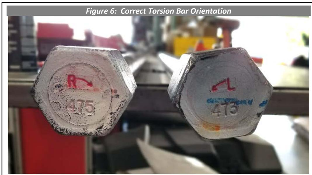
11. Install the torsion bars the same way the OEM ones were removed. Now install the key in the same position it was removed noted in step 8. Use the hammer and punch to tap the bar in to place until it reaches the end of the torsion key compartment but has a small gap (See Figure 7).
