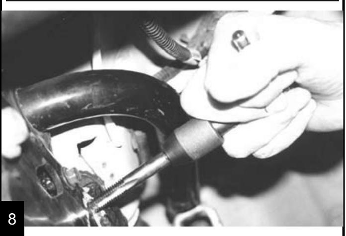
Push the link onto the frame stud, this will provide a guide for the pin position install on the other side.
