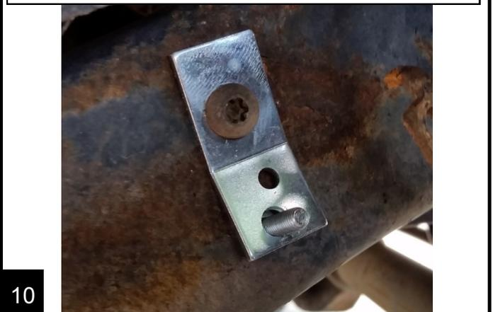
Using the supplied 1/4" nut and bolt, secure the factory bracket to the new bracket.
