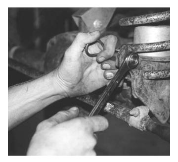
**Step 4**Attach the sway bar arm by sliding the polyurethane bushing onto the lower stainless steel stud. The use of lubricant such as WD-40 will make this much easier.
