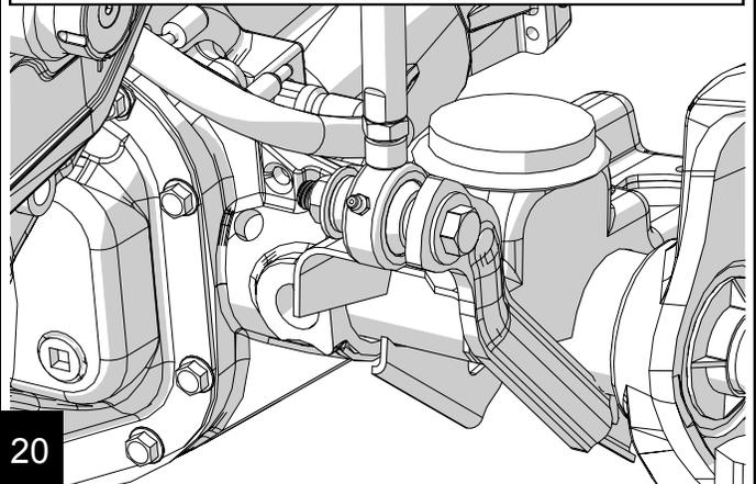
Lengthen the links so the forged sway bar arms are angled up slightly. The ends of the links are right and left hand threads. Simply twist the tube to adjust the length similar to a turn buckle. Adjust the link lengths so the engagement knob engages and disengages easily.
