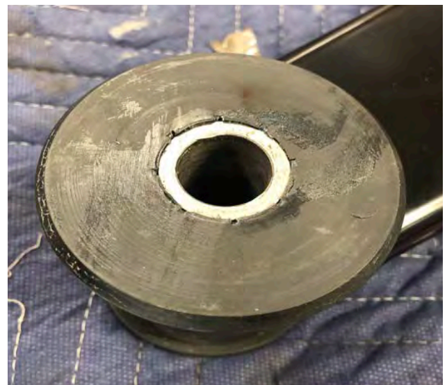
Figure 24: Crush Sleeve Installed
