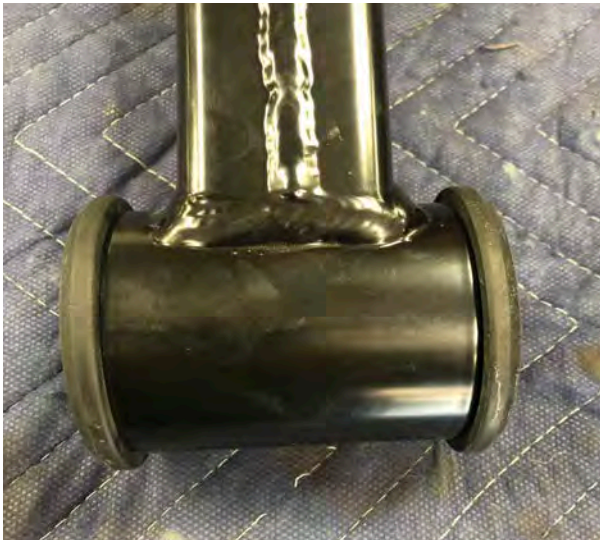
Figure 21: Traction Bar Bushings Installed
