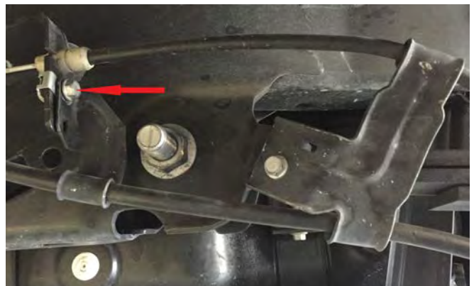
Figure 2: Brake Cable Bracket Mounting Bolt
