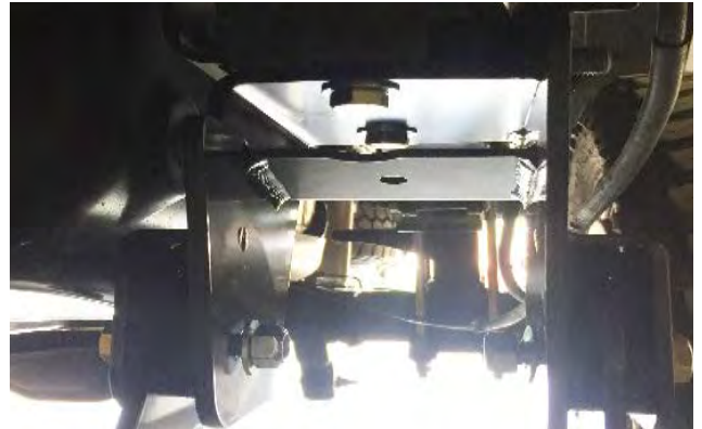
Figure 10: Front Mount Installed
