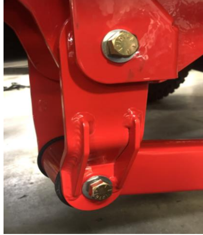
Figure 32: Traction Bar / Shackle Pivot
