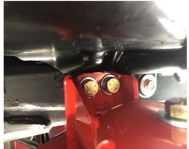
Figure 13: Fuel Tank Shield Trimmed
