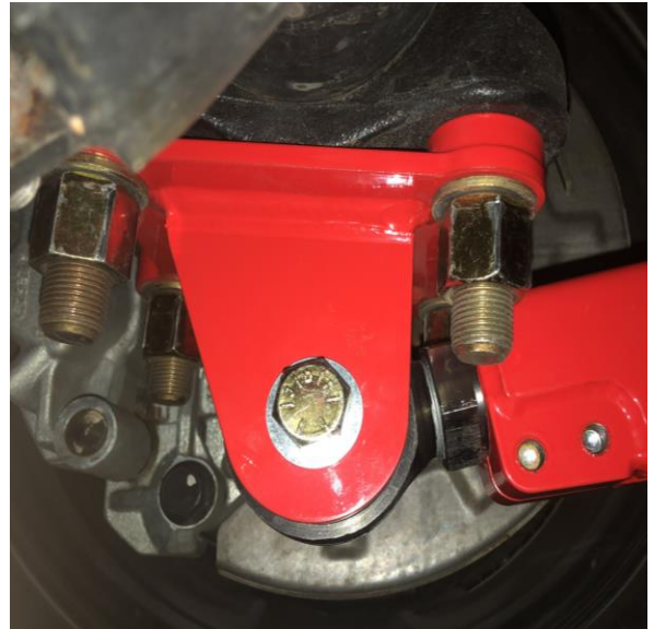
Figure 35: Traction Bar Rod End / Rear Axle Pivot
