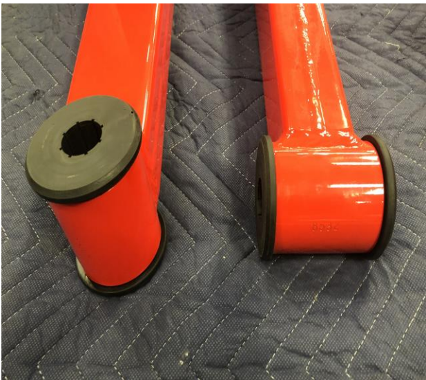
Figure 28: Traction Bar Bushings Installed
