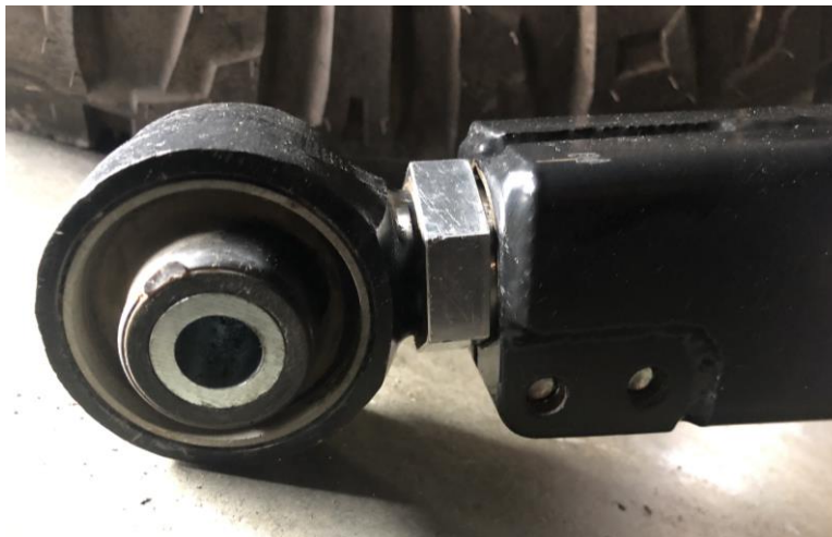
Figure 26: Traction Bar Rod End
