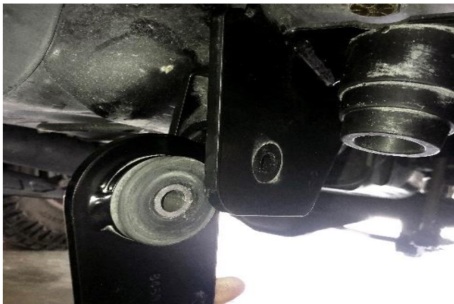
Figure 16: Assemble Shackles to Frame Mount
