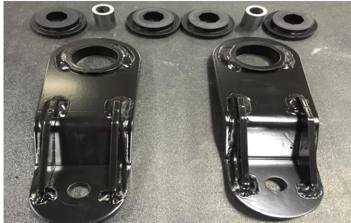
Figure 11: Traction Bar Shackle Parts
