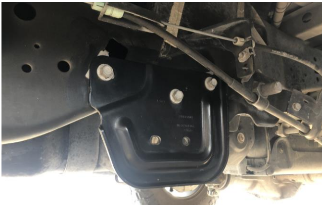
Figure 1: Fuel Tank Stone Deflector
