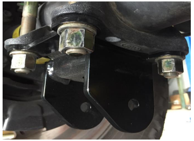
Figure 19: Install Axle Mount Bracket
