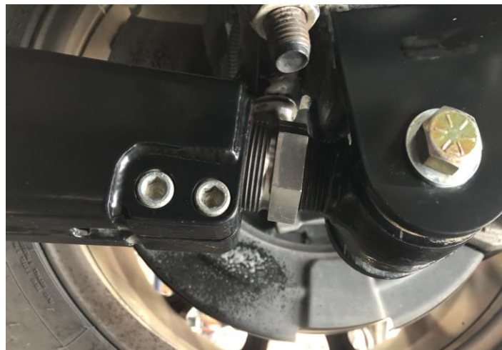
Figure 29: Adjuster Nut Clamp
