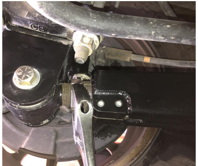
Figure 28: Traction Bar Rod End / Rear Axle Pivot
