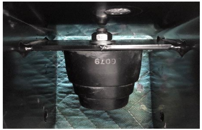
Figure 8: Bump Stop Mounting Nut
