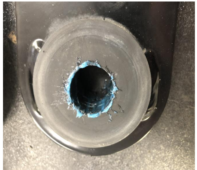
Figure 13: Grease Shackle Bushings
