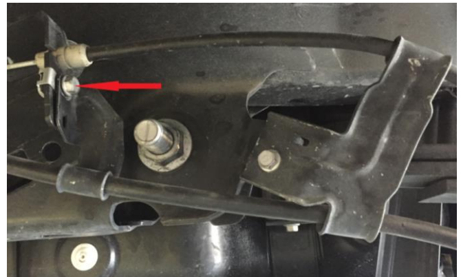
Figure 2: Brake Cable Bracket Mounting Bolt
