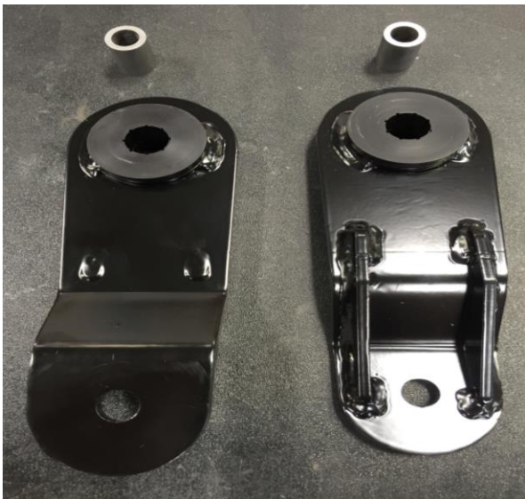
Figure 12: Install Shackle Bushings
