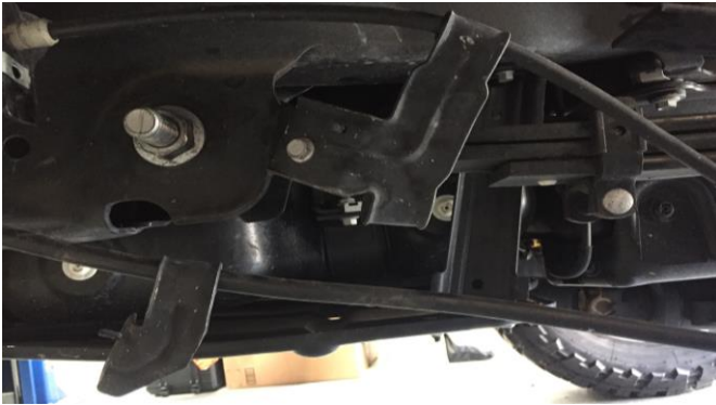
Figure 3: Brake Cable Removed
