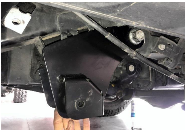
Figure 5: Frame Mount Bracket Alignment
