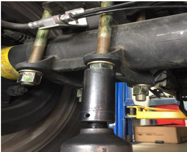
Figure 18: Remove U-Bolt Nuts
