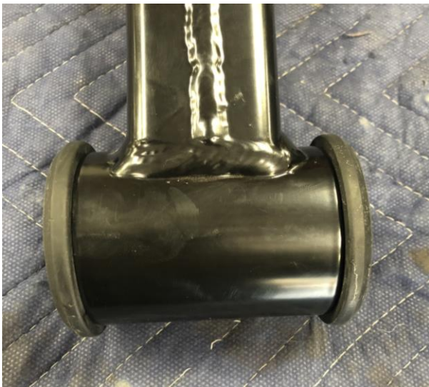
Figure 21: Traction Bar Bushings Installed
