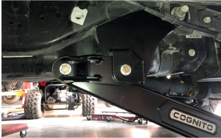
Figure 25: Traction Bar / Shackle Pivot
