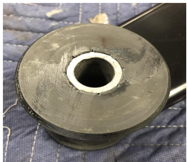
Figure 24: Crush Sleeve Installed
