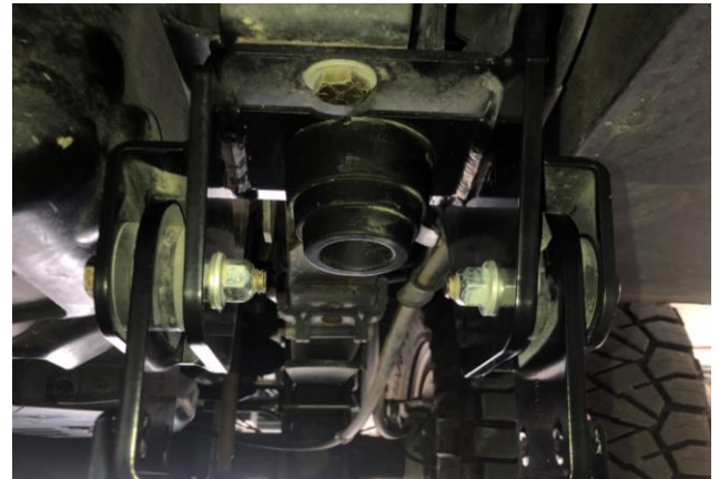
Figure 17: Frame Bracket Assembled
