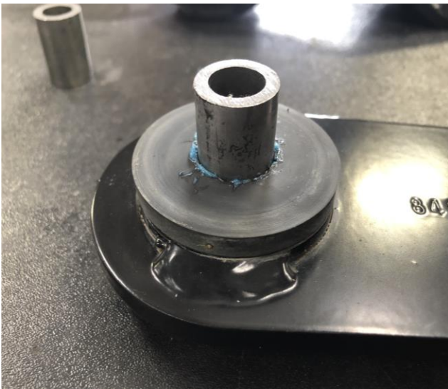
Figure 14: Install Shackle Crush Sleeves
