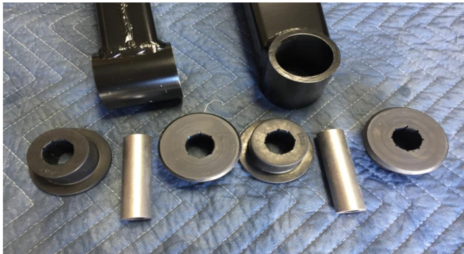
Figure 20: Traction Bar Bushing Parts
