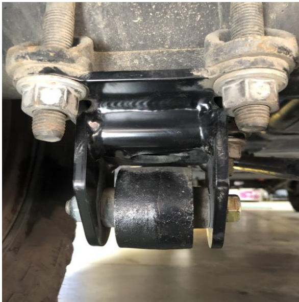
Figure 27: Traction Bar Rod End / Rear Axle Pivot
