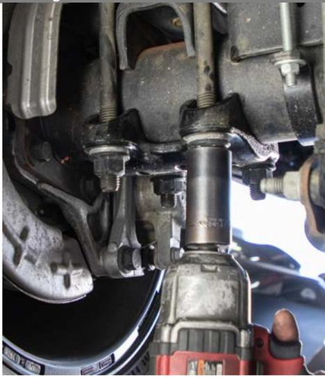
Figure 18: Install Axle Mount Bracket
