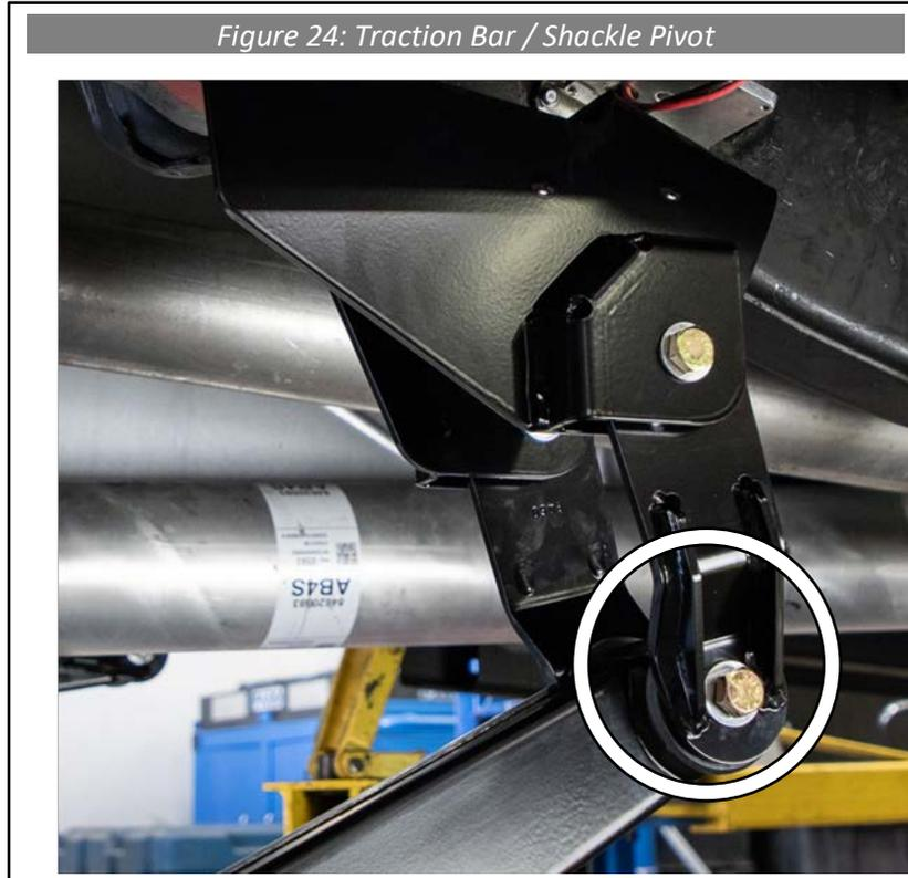
18. Insert the traction bar rod end between the eyelets on the rear axle mount. Notice that the tubular traction bar has a flat section about 6" from the forward end. Make sure the flat section (bump stop pad) is on top. Turning the adjuster sleeve only, lengthen the traction bar tube until the rod end lines up with holes in the traction bar mounting eyelets. Install using the hardware listed below found in **HP9205** and tighten to 120 ft. /lb. using a 7/8" and 13/16" wrench (See Figure 25).
