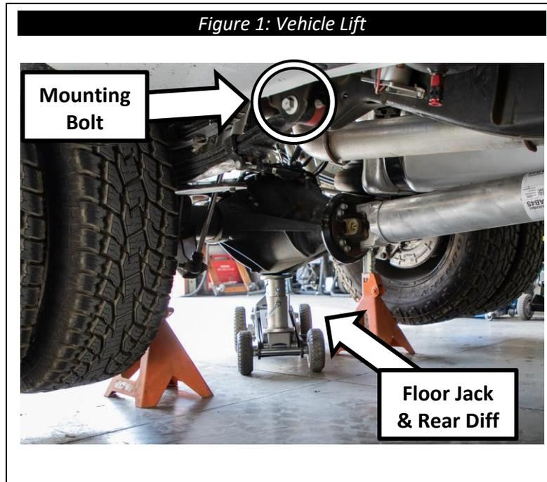
3. Remove the forward leaf spring mounting bolt using an impact with a 24-mm socket. Place the hardware safely aside, it will be reused later.
