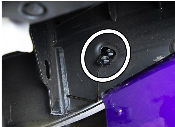
9. Locate **HP9205** and find the two (2) 1/2" flat washers, two (2) 1/2" lock washers, and two (2) 1/2"-13 x 1.25" bolts. Install the lock washer between the flat washer and the bolt head and bolt the frame mount bracket to the nut plate, see Figure 6. Tighten and torque these two (2) bolts to 90 ft-lbs.
