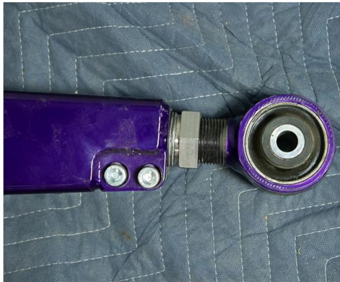
20. Locate **HP9205** and find one (1) 9/16"-12 x 5" bolt, two (2) 9/16" flat washers, and two (2) 9/16"-12 lock nuts. Install the traction bar end with the bushings between the frame mount bracket shackles, see Figure 15.
