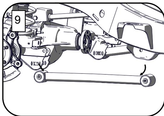
13. After all the control arms are installed, and the Jeep is sitting at ride height, torque the front and rear track bar bolts to 125 ft-lbs.
